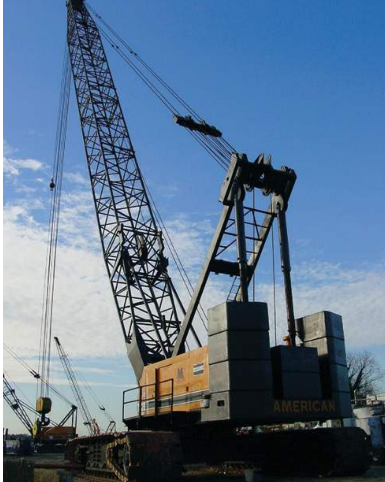
American 450-ton capacity crane
